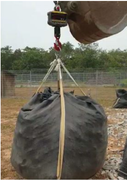
Figure 14: The weight of the sinkers is checked with a weighing scale on a crane hoist.
