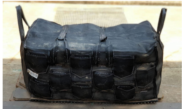
Figure 3: GeoBags made of 100% monofilament polypropylene engineering fabric
